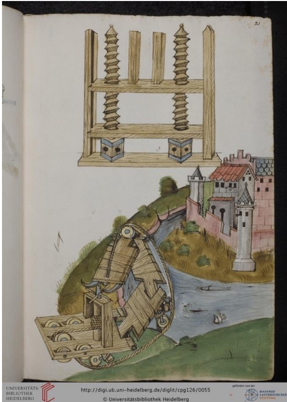
Fig. 5. Mönch, mechanism for laying a bridge from one side. Heidelberg, Universitätsbibliothek Heidelberg, Cod. Pal. germ. 126, fol. 21r. Courtesy of University Library Heidelberg (public domain).
