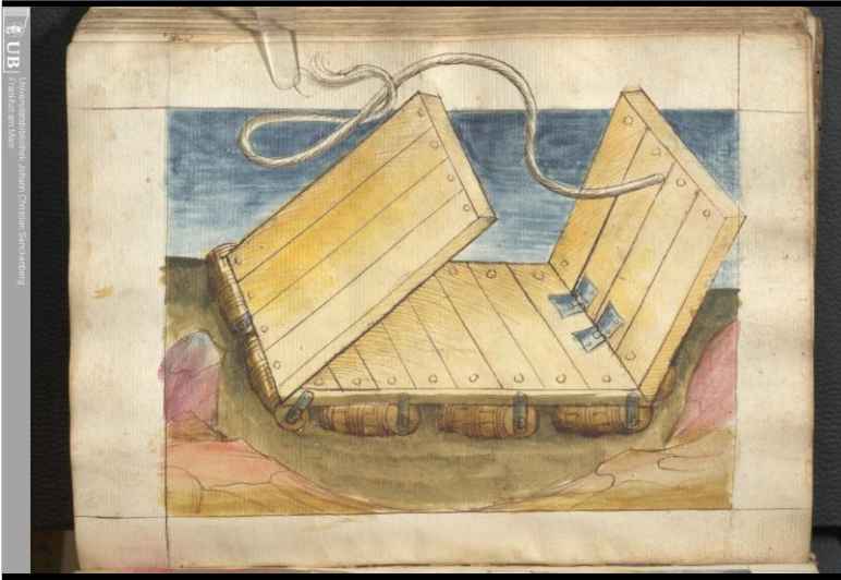
Fig. 2. Bellifortis, raft to be placed into a ditch, with fold-out ramps. Frankfurt a.M., Universitätsbibliothek J.C. Senckenberg, Ms. germ. qu. 15, fol. 120 v /p. 242. Courtesy of University Library J.C. Senckenberg, Frankfurt a.M. (public domain).
